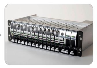
The *ViaLiteHD* wide dynamic range broadband fibre optic links have 0dB link gain. For installations where the number of cross site fibre connections is limited the complete ITU range of CWDM transmitter wavelengths is offered allowing up to 18 channels to be carried on one fibre. Optical connector options include FC/APC, E2000/APC and SC/APC.
