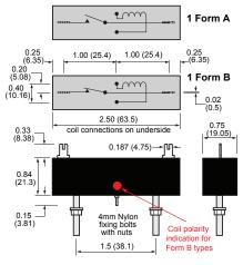
Important: For all Form B types, the correct coil polarity must be observed. The positive connection is shown by the red spot on the package
