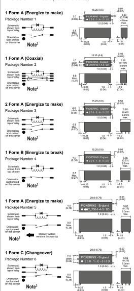
Note<sup>3</sup>: When an optional diode is fitted the orientation spot end of the relay forms the positive connection.
