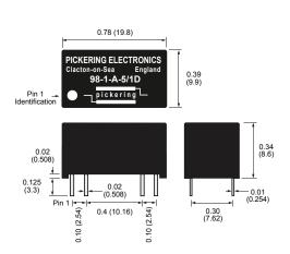
Schematics are shown from UNDERNEATH the relay.
