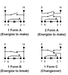
Important: Where the optional internal diode is fitted or for all Form B types, the correct coil polarity must be observed, as shown by the symbol on the schematics.
