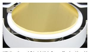
MPI Non-thermal Triaxial High Power Chuck with gold plated surface for low contact resistance
