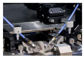
Off-axis wafer alignment camera
