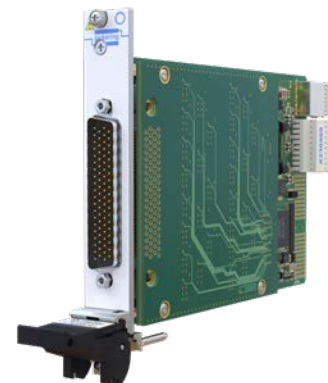
42-739-001 MIL-STD-1553 Single 16-Channel, 2-Pole Multiplexer (PXIe Version)
