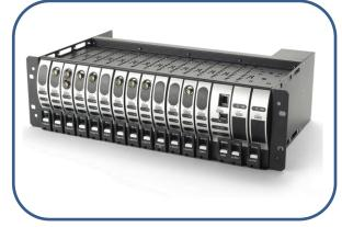
The IF modules are finely tuned to provide a superior dynamic range and a flatness of 0.2dB across the full band. Chassis modules have gain change ability to support better performance and overcome more optical loss in the fiber link by adjustments made in either manual gain control, software gain control or automatic gain control through the SNMP module.
