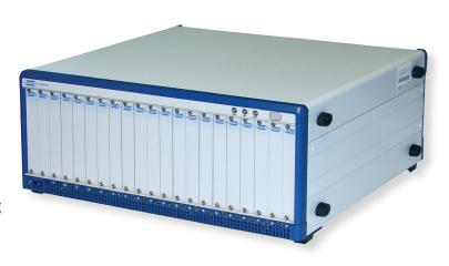
An intelligent chassis management system monitors the power supply voltage, internal temperature and the cooling fan speed. The current condition of the chassis is displayed on front panel status LEDs and can also be monitored remotely via an RS232 port
